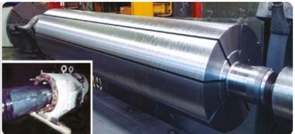
Compressor cylinder before and after restoration
